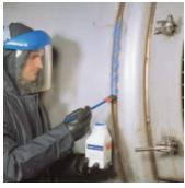
80% fume reduction compared to standard Pickling Paste.
